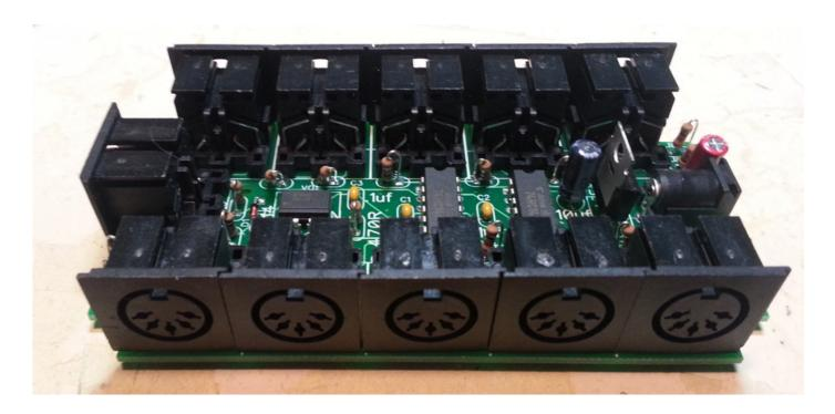
to heat one pin and then reseat the jack. Now I solder the remaining pins. Do the same for the five jacks on the other side and you are done.
