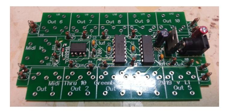
Once those are soldered and clipped, we add the jacks. I add the Midi In jack first as this lets the board sit balanced upside down with the Midi In jack on one end and the Power regulator on the other.
