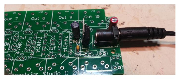
Once those parts are on, I go ahead and plug it in and test for the correct 5 volts. The heat sink on the regulator is gound and the top right hole on the 74HC14 is +5. If this measures correctly, time to add the rest of the components.
