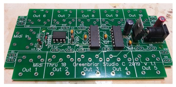
Note that the two resistors are placed on end, so to speak. In order to get ten outputs into as compact a box as possible, all the resistors are placed by folding one lead back along the resistor body and placing it on the board standing up from the board.
